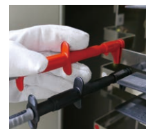
For clamping around the target busbar
